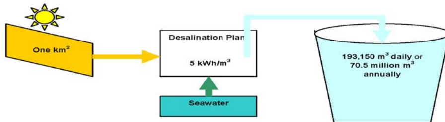
Figure 7a. Relationship between solar collector area and the amount of desalinated water it can produce
